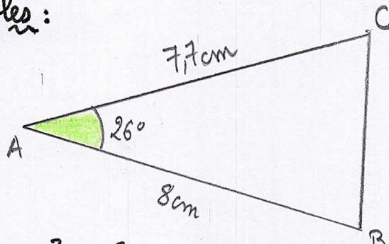
$$\begin{aligned} BC^2 &= AB^2 + AC^2 - 2 \times AB \times AC \times \cos(\hat{A}) \\ &= 8^2 + 7,7^2 - 2 \times 8 \times 7,7 \times \cos(26^\circ) \\ &\approx 12,59 \end{aligned}$$
